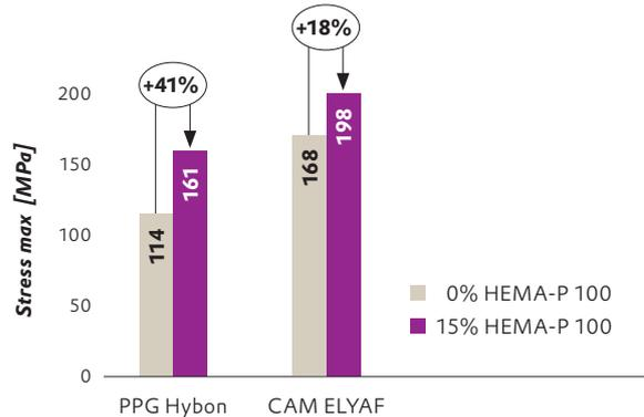
Figure 4 provides the results of the compression testing of laminates containing **VISIOMER® HEMA-P** as strength promoter versus the standard UP resin without strength promoter. The measurements confirm again the improvement of mechanical properties using **VISIOMER® HEMA-P**. The performance increase depends on the glass fiber type. The increase of compression strength in 90° direction for PPG HYBON 2002 is up to 41%, where the increase for CAM ELYAF WR6 is lower but still significant at 18%.
