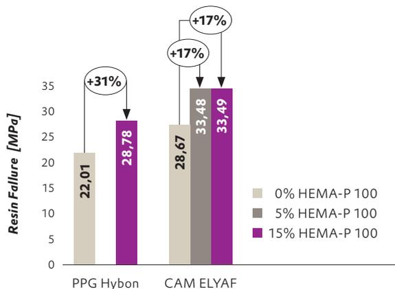
Figure 3 shows the resin failure of the different resin formulations taken from the 90° tensile testing. In contrast to the ILSS measurement, the increase in resin failure
